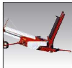
The Intake Transfer Hopper folds back over the main drive assembly during transport.
