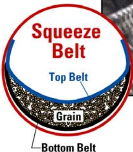
The gentle squeeze of the bottom and top belts convey more volume up steeper inclines with less product damage.
