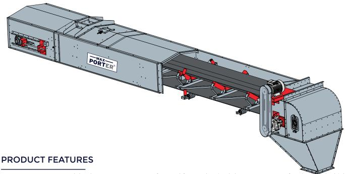
Our Maxporter R Model Belt Conveyors are manufactured from galvanized sheet. Its upper surface is closed which makes it to be able to work in outdoor conditions. In this way, it is a long-lasting equipment against environmental factors. This type of our belt conveyors uses less energy due to its carrier rolls. Our anti-static belts are resistant to the risk of fire and dust explosion.
