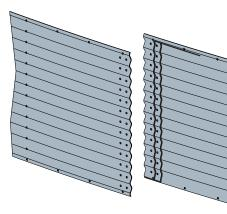
Heat and cold-resistant strip mastics, used in the joints of wall sheets, ensure perfect sealing in all types of climates.
